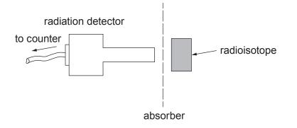
The following table shows how the count rate for four different radioisotopes is affected by different absorbers.
